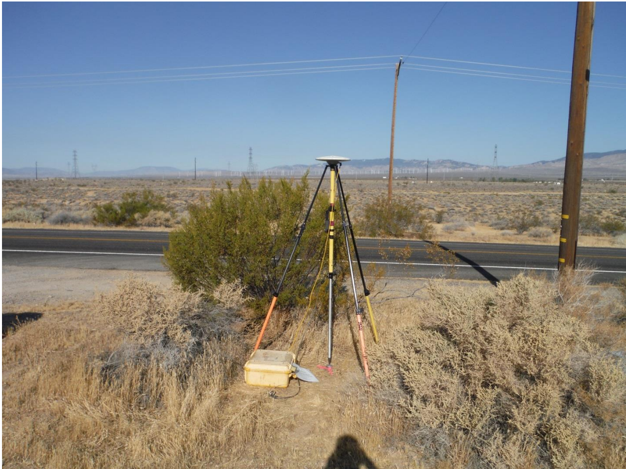
Figure 4: A photo taken by the QSI acquisition team of a Trimble R7 base station set up within the California High Speed Rail South AOI
