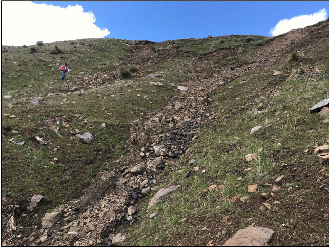
Photo E: Debris flow deposits down gradient from main landslide mass. Note debris flow in foreground originating from main debris slide mass; note active water flow from seepage at source in debris slide face. The channel gradient is approximately 30 degrees.
