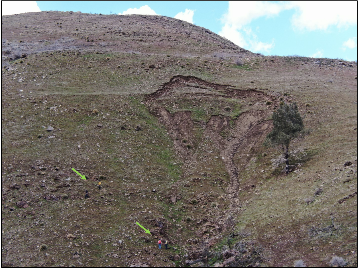
Photo B: View north of Cane Peak landslide; note CGS and Kern County staff for scale (denoted with green arrows). Note benches at and above head of March landslide, which likely formed due to past movement of older, larger landslides. Also note debris flow tracks down slope originating from main debris slide mass. Drone photo provided by UC San Diego.
